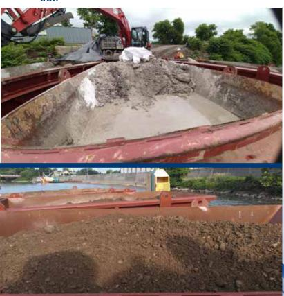
The Poseidon Dredge / Rock Box is designed for heavy duty use on your construction projects. Designed to hold dredging spoils from Mechanical Dredging, the Poseidon Dredge Box can be loaded & off loaded with an excavator or picked with a crane using the (4) built in pick points. The box can be emptied by disconnecting two of the crane lines and dumping out the box or with the excavator bucket.
