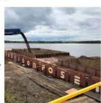
The Poseidon Hopper Barge is made to the same dimensions as the standard barge section. The P2-7' Hopper has male and female connections to allow for the sections to attach to one another or to other Poseidon P2-7' barge sections.
