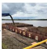
The Poseidon Hopper Barge is made to the same dimensions as the standard barge section. The P2-7' Hopper has male and female connections to allow for the sections to attach to one another or to other Poseidon P2-7' barge sections.
